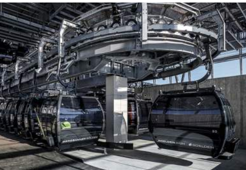
The Giggijoch Gondola has been built with Doppelmayr's D-Line technology and can transport 4,500 pphpd (highest capacity for a MDG system)
